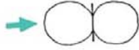
Dipole antenna picks-up signals from both the front and rear equally well.
